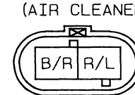
B2-40 ENGINE COOLANT TEMPERATURE SENSOR (EM2)
