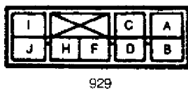
Fig. 4: Main Switch Connector Terminal ID Courtesy of Mazda Motors Corp.
