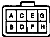
Fig. 59: View of Solenoid Valve Connector Courtesy of Mazda Motors Corp.
